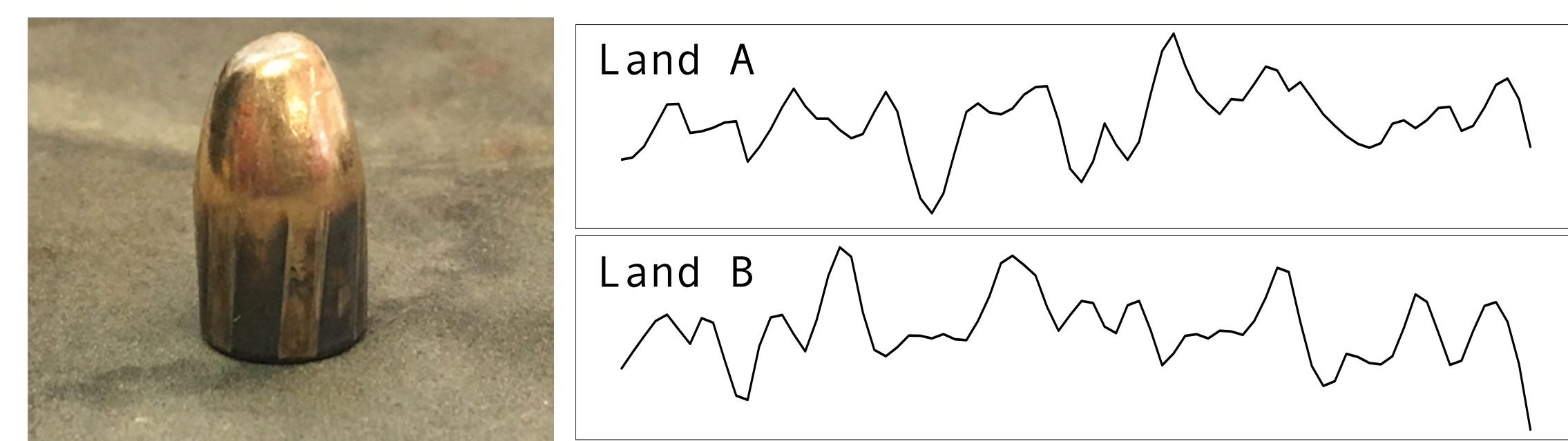
Figure 1: The picture on the left of a bullet shows the alternating land and groove impressions created when the bullet is fired from a gun. The raised portions are referred to as lands. The image on the right shows a representation of the comparison of two signatures obtained from the scans of bullet lands.
